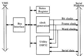
On this card, the host can write registers that set the serial receive and transmit rates for all the processor modules. It also generates the clock for the processors. As mentioned above, a DSP-32 serializes data from the host and put it on reserved address 0. It can also read from any address.
