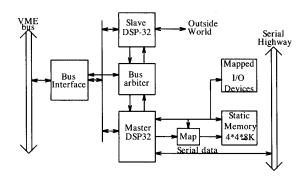
There are two DSP-32s per "processor module". The "master" (with external memory) is connected to the serial lines going to and from the crossbar switch. The "slave" is connected to external I/O devices such as A/D and D/A converters. It is responsible for vari-
